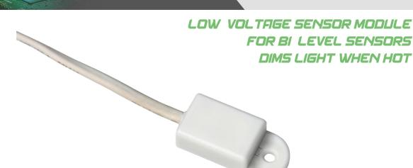
**WEC-2TS** is an innovative and intelligent temperature management sensor. It helps preserve the LED life of highbays and other fixtures with dimming drivers. It is powered by the common 0-10V interface without the need for an extra power supply. Attach this sensor on the LED board of the fixture and it will reduce the output power of the LED driver to 50% when the temperature reaches 160°F. It will maintain the light output at 50% until the board cools down.
